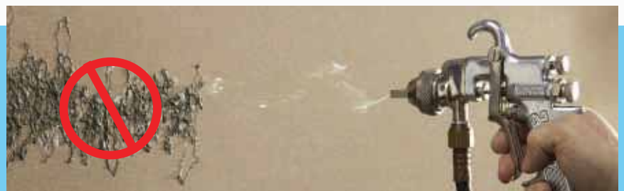
Controlled spray eliminates waste associated with puddling, "fire hosing," and uneven stringing pattern (shown above).
